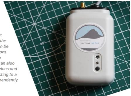
**Extending Checkmate features** - Checkmate is a reference design Smart device and extension to the Pulse Online Cloud. It can be extended with new sensors, processing logic or radio modules. Our software can also be used in other PLC devices and microcontrollers, connecting to a network or running independently.
