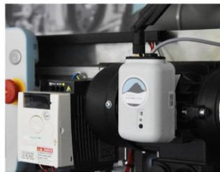
**General machinery** - Install in difficult to reach places, moving operations or dangerous spots and safely monitor from anywhere. Checkmate can use an accelerometer to detect motion and easily by report abnormal movements.
