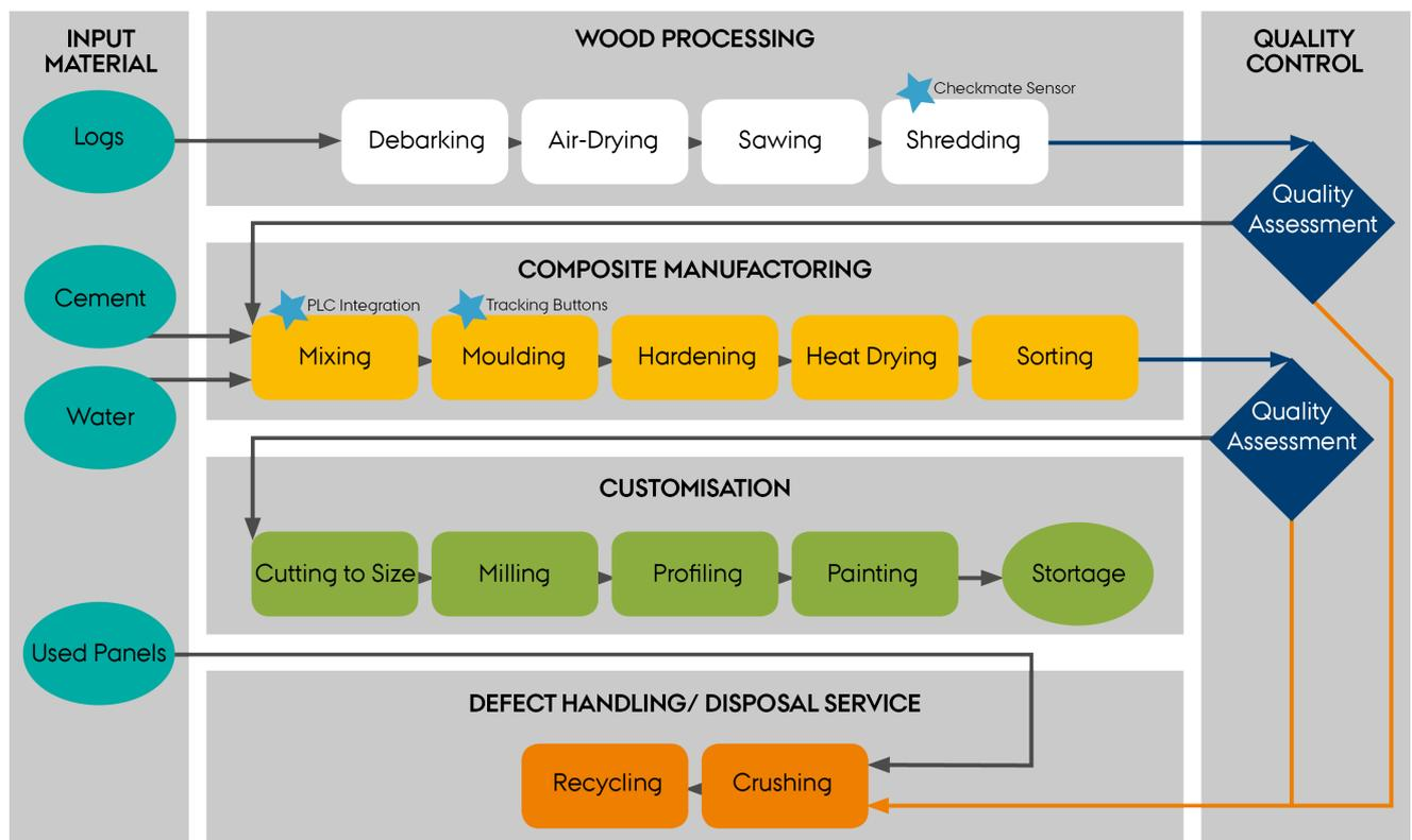
Figure 1: Troldekt's production process. \* indicates where the IIoT project through its lifetime applied new technology.
